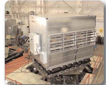
California's building code mandates OSHPD certification of critical care equipment—including air handlers. The combined efforts of The VMC Group (certified seismic qualification agency), Clark Dynamics and Trentec (certified independent testing laboratories), and Temtrol engineers, has resulted in OSHPD pre-approval for Temtrol Series ITF. Five frame sizes of Series ITF construction endured shaker table testing with no flaws or engineering changes required to the standard construction.
